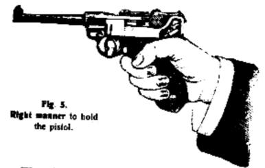
Therefore hold the pistol firmly pointed at the target so that the automatic safety sear (29) projecting from the rear of the stock is pressed in. To fire the pistol, pull the trigger (20) and release it again as long as the cartridges
